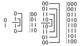
These characteristics suggest a simple and fast method of translating a binary value into the corresponding BRGC. Each bit is inverted if the next higher bit of the input value is set to one. This can be performed in parallel by a bit-shift and exclusive-or operation if they are available. A similar method can be used to perform the reverse translation, but the computation of each bit depends on the computed value of the next higher bit so it cannot be performed in parallel.
