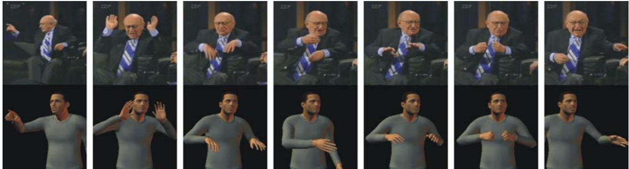
Figure 1. Selected frames of a source video (top) and a kinematic animation (bottom). The animation re-created the motion of the gesturing arm/hand of the original video from a manual annotation of the video which is based on our annotation scheme.
