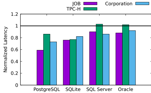
Figure 9: Latency of test query plans created by Neo after 100 episodes of training, normalized to plans created by the target system’s corresponding optimizer for different workloads.
